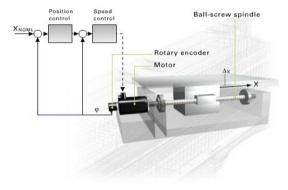
> **Semi-Closed Loop** One position feedback for speed and position control
