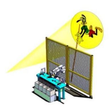
**ISO/DIS 14120** type-B2 standard (General requirements for the design and construction of fixed and movable guards)
